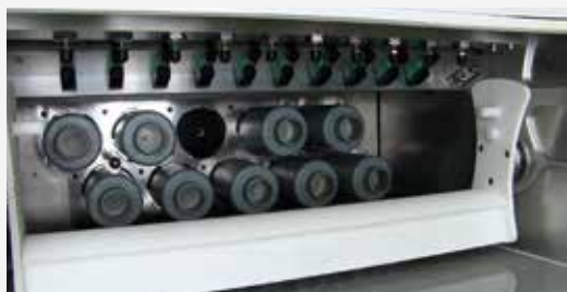
↑ Waste shot collector array
