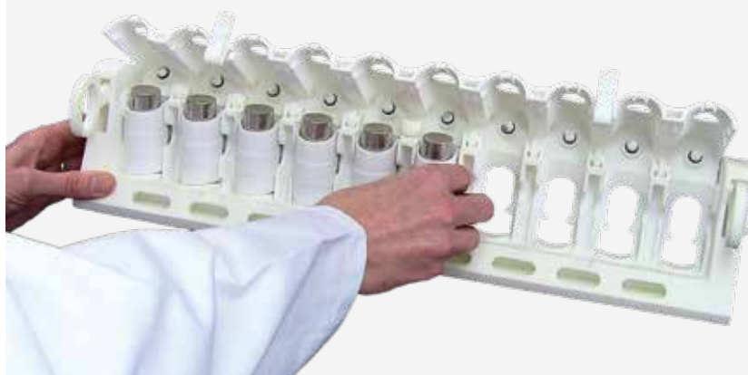
↑ Placing MDIs into carriage
