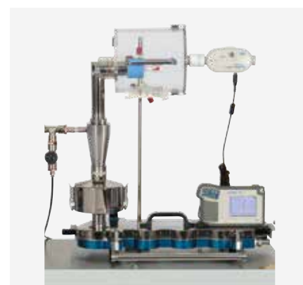
Real Time Breath Profile Verification Chamber (with inhaler in situ during test) supported by the Accessory Support Stand on the Breathing Simulator BRS 3100
