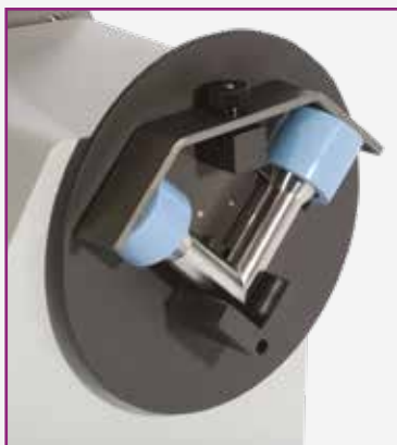
↑ Fixture with NGI Induction Port
