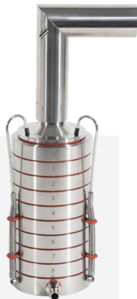
↑ Anderson Cascade Impactor (28.3 L/min Version) with USP Induction Port
