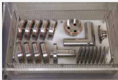
↑ ACI Carrying Rack in Rinse Bath
