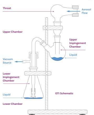
The GTI operates on the principle of liquid impingement to divide the dose emitted from the inhaler into respirable and non-respirable portions.
