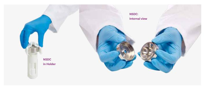
With an opening large enough to prevent splashback, but small enough to greatly reduce the risk of drips and leakage, the NSDC not only ensures accurate collection of the full dose, but also enables dose collection to occur in a vertical orientation to better replicate
