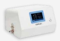
Ensuring that the volume of air sampled does not exceed the pharmacopoeial specifications, the Breath Actuation Controller BAC 100i contains an electronically operated, timer-controlled two-way solenoid valve and is positioned between the impactor and Vacuum Pump to control air flow through the inhaler.
