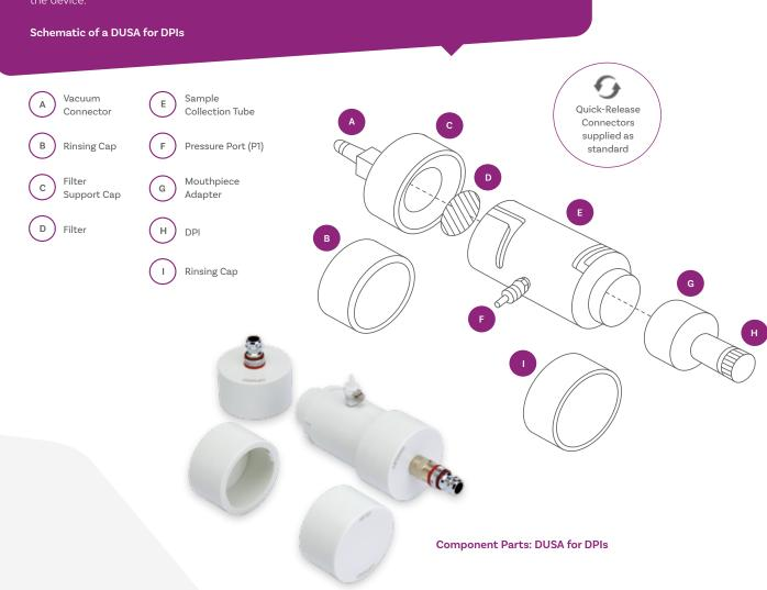
During testing, air is drawn through the sampling apparatus to broadly simulate inhalation. A critical flow controller is required to control air flow supply to the inhaler and ensure critical (sonic) flow conditions during testing.
