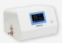
Ensuring that the volume of air sampled does not exceed the pharmacopoeial specifications, the Breath Actuation Controller BAC 100i contains an electronically operated, timer-controlled two-way solenoid valve and is positioned between the impactor and Vacuum Pump to control air flow supply to the inhaler.
