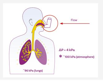
It is this Flow Rate Q, that the pharmacopoeias state should be used for DDU testing and APSD measurement.
