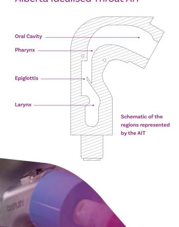
For orally inhaled products (OIPs), the AIT provides analysts with data more representative of measured *in vivo* behaviour, by ensuring that the ISM corresponds with the portion of the aerosol that would likely enter the lungs.
