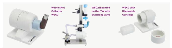
The Waste Shot Collector WSC2 is a compact vacuum filtration system suitable for use with a range of devices. It can be used in either standalone mode or integrated into the Inhaler Testing Workstation™ ITW (see page 204), via a switching valve, whereby the vacuum pump used for the DUSA powers both sampling and waste collection units.
