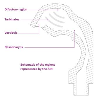
Understanding and optimising regional deposition is essential to maximise the fraction of drug absorbed via the target pathway and to minimise drug transit to the lungs. For nasally inhaled products, the AINI enables representative testing of the deposition of drug within the nasal airways.
