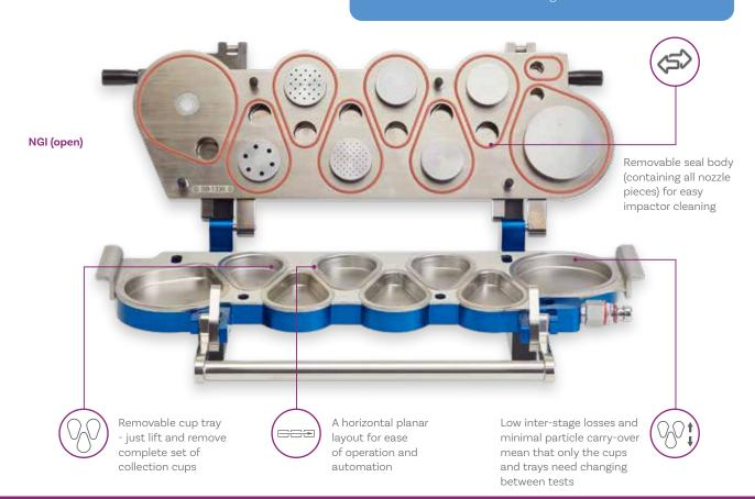
The sample-laden air flow passes through the NGI in a saw-tooth pattern across stages arranged in a horizontal plane.
