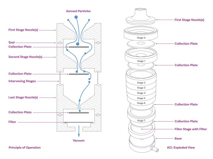
Unlike the NGI, the stages of the ACI are arranged vertically. The aerosol flow passes first through the stage at the top of the impactor, through to the last stage and a final filter at the bottom of the impactor arrangement.
