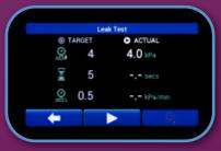
Leak test screen
